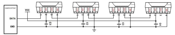
Remarks: According to the quality of power supply, please connect a filter capacitor in parallel between VDD and GND, the recommended value is 100nf.
